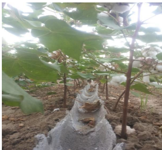
Fig. 3. Practical application of the obtained porous material from phosphogypsum to reduce the irrigation rate.
