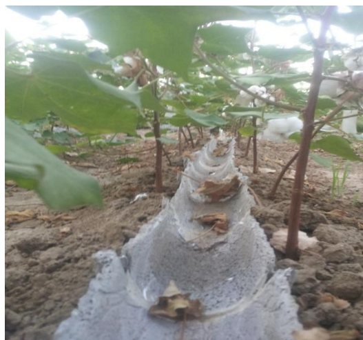
Fig. 3. Practical application of the obtained porous material from phosphogypsum to reduce the irrigation rate.
